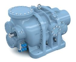
The GEA Grasso LT series comes in fourteen sizes and covers a swept volume from 805 to 8560 m³/h. Due to the combined sleeve and roller bearing of the rotors, the compressor has an extremely long life span and low noise and vibration levels. All components are designed for long operating life, high availability and easy maintenance. Furthermore, the compressors of the GEA Grasso LT can be provided according to the API 619 standard and ISO 10440, respectively.
